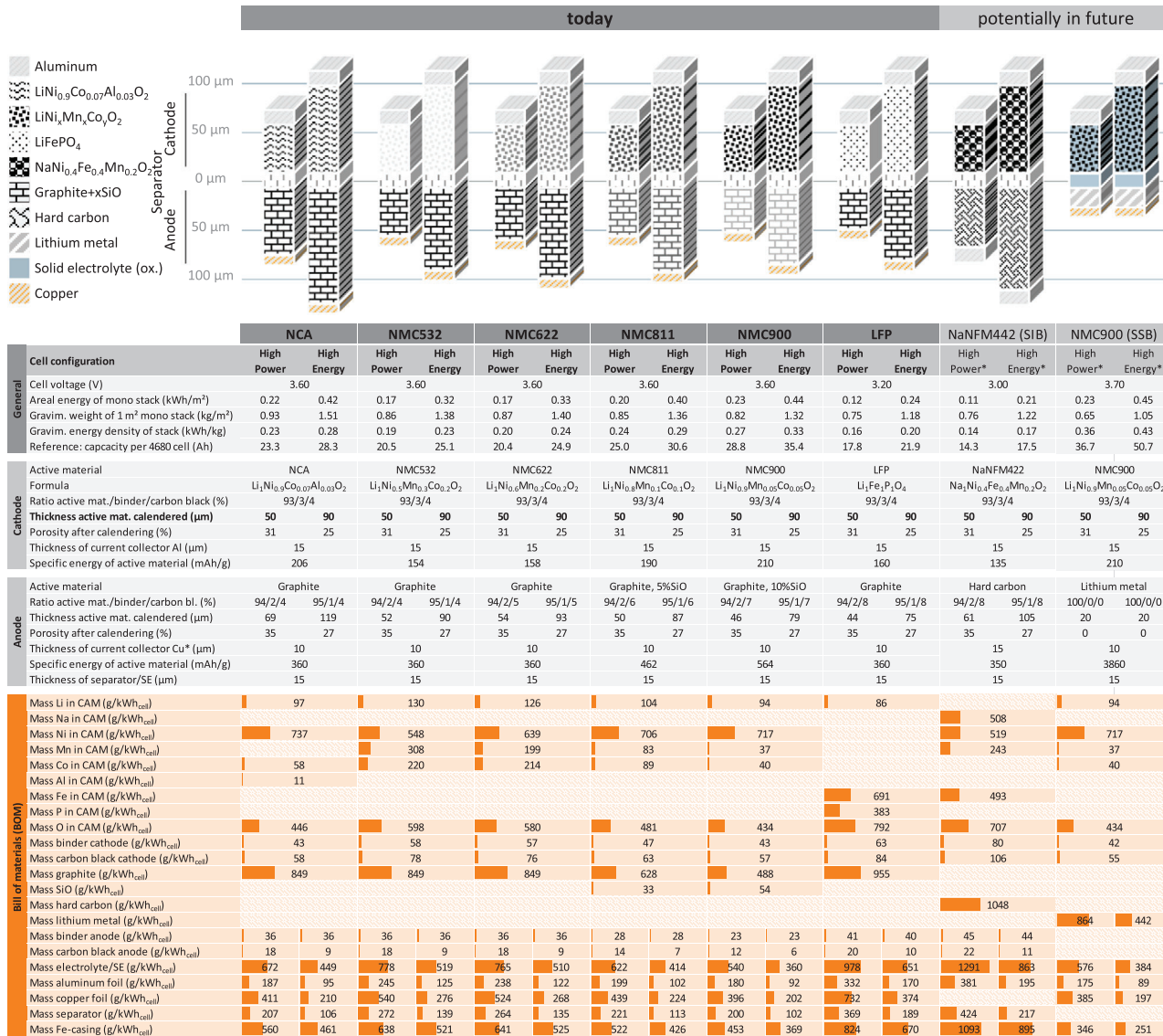
FIGURE 3 Stack designs and bill of materials of current lithium-ion battery (LIB) cells in electric vehicles (EVs). The cells are designed based on product teardowns of automotive battery cells (A2Mac1, 2023; Quinn et al., 2018), on battery databases (Fraunhofer Institute for Systems & Innovation Research ISI, 2023), and on meta-studies that investigate automotive battery cell designs between 2016 and 2022 (Link et al., 2023); >67% of the analyzed LIB cells in EVs have a cathode coating thickness between 50 µm (high-power [HP] configuration) and 90 µm (high-energy [HE] configuration), (n = 75) (Link et al., 2023). Calculations and further details can be found in Supplement S2. We use Li 1.3 Al 0.3 Ti 1.7 (PO 4 ) 3 as a solid electrolyte for the solid-state battery (SSB) cell. *Whether a distinction between HP and HE cells will be made with sodium-ion batteries (SIBs) and SSB in the future is unknown, but for better comparability, we designed both chemistries once in an HP and once in an HE configuration. LFP, lithium-iron-phosphate; NCA, nickel-cobalt-aluminum; NMC, nickel-manganese-cobalt.
