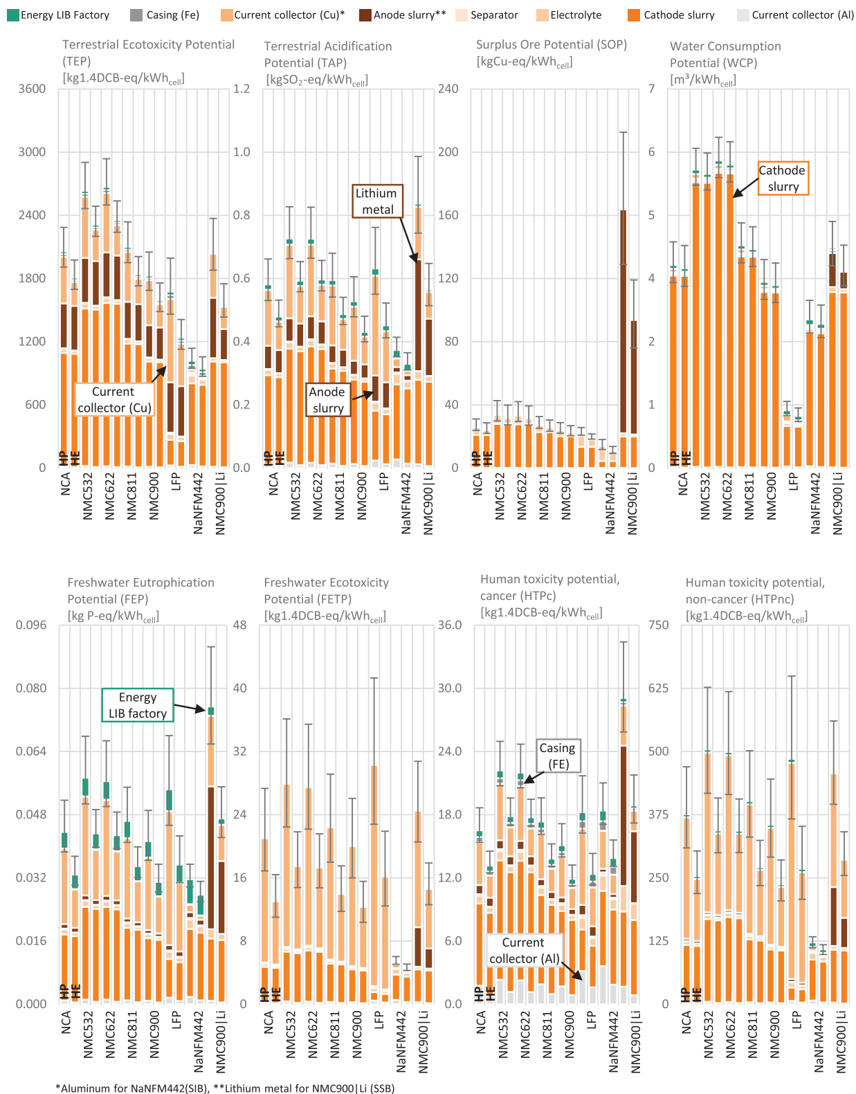
FIGURE 7 Environmental impact of different LIB chemistries, in different configurations. The corresponding data can be found in Supplement S2. The data have a log-normal distribution. The error bars show the approximated 67% confidence interval. HE, high energy; HP, high power; NMC, nickel–manganese–cobalt; LFP, lithium–iron–phosphate; NCA, nickel–cobalt–aluminum.
