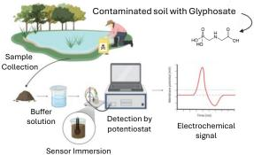
The sensor interacts with the sample for a few minutes, measuring the electrochemical signal in real time, making it possible to identify and determine the concentration of pollutants.
