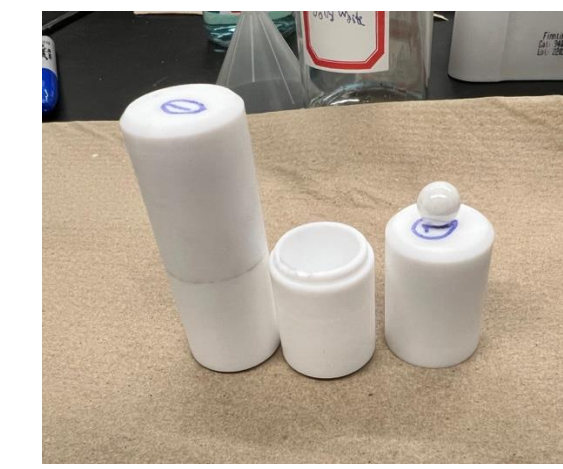
Teflon Milling Jars and Zr Infused Ceramic Balls
