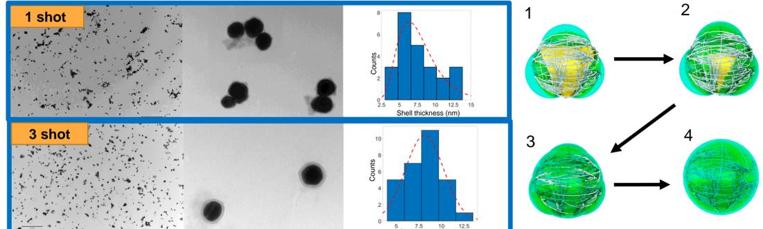
TEM micrographs of gold and titanium dioxide core-shell nanoparticles with a shell of different thickness
