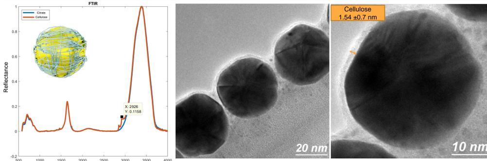
ATR-FTIR spectrum of AuNPs, with sodium citrate and cellulose as stabilizing medium
