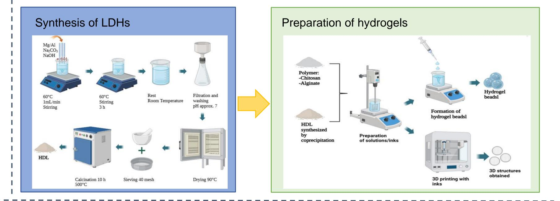
hydroxides (LDHs), are effective adsorbents for contaminants such as nitrates. In this study, hydrogels incorporating LDHs were developed to create filters for water remediation. Synthesis, characterization, and nitrate removal tests were performed, achieving good results in both simulated and real water. Subsequently, a composite material of LDHs and biopolymers (alginate) was fabricated into spheres and 3D structures, which were tested as adsorbent materials.
